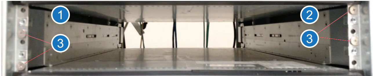
Figure 14: Rail Attachment to Front of Rack (screws fastened to back of rack post - facing rearward)
